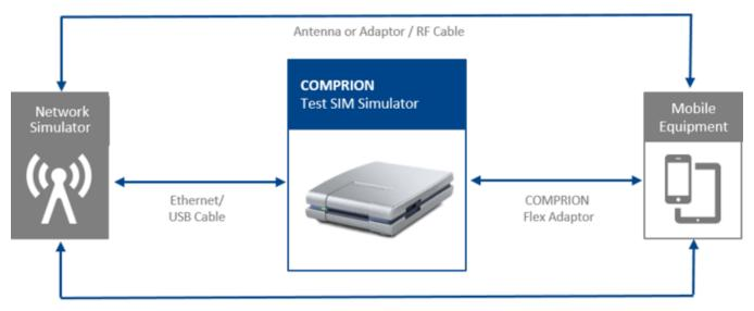
Connection for Automation of the Mobile Equipment
